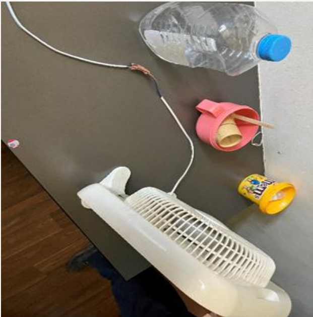
Modified lengthen wiring from fan and electric cable holding door open
